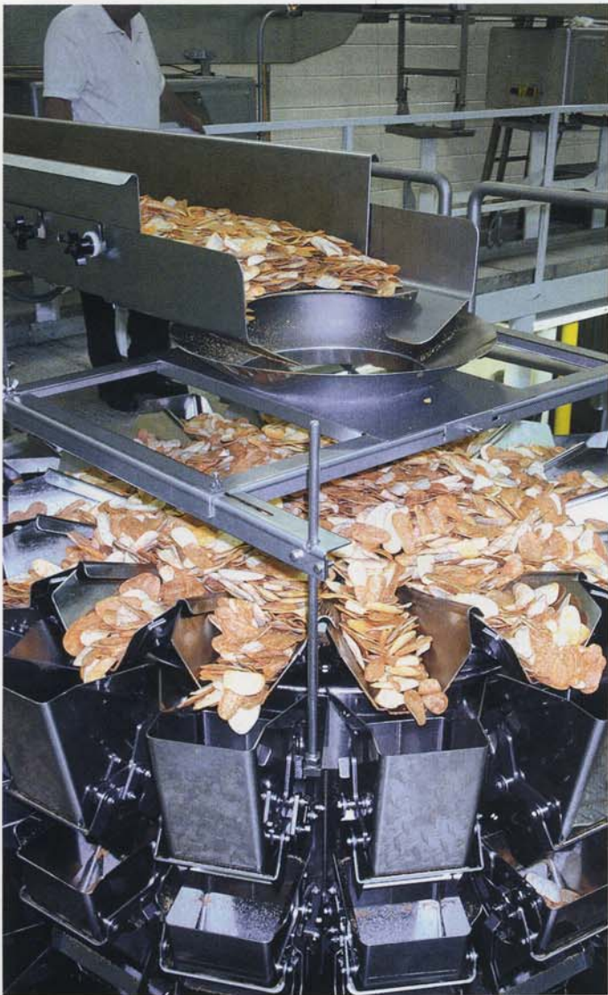
The bright bags, top, communicate a lively chip experience from the T.G.I. Friday's products. A 16-head rotary scale, above, weighs the Cheddar and Bacon Potato Skins before they move to a continuous hf/f/s machine.
