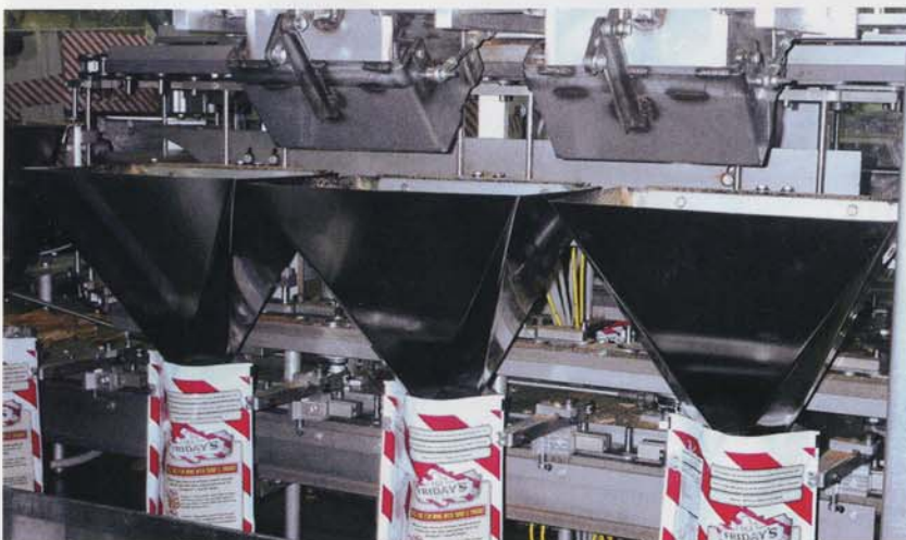
Ten funnels rotate around an oval racetrack filling the 7.5-oz bags, two at a time.
