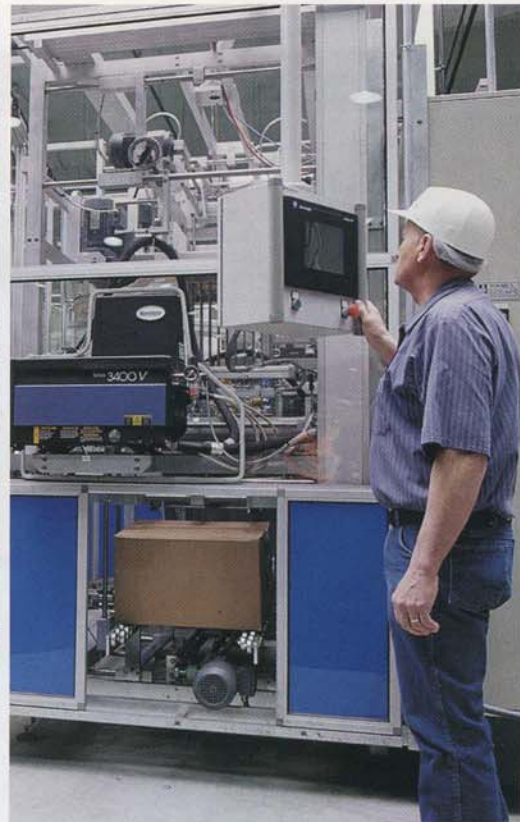
Automated wraparound case packing system is designed specifically for stand-up pouches and saves up to 50 percent on costs of shipping/display boxes, transportation and handling.
